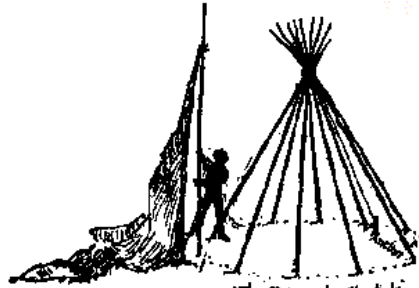
2 nd Set up tenth pole with (sheet) cover fastened to it by lark rope
