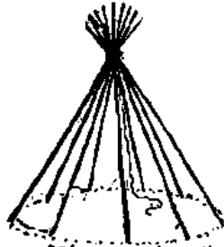
3 rd Set up wind other six poles
